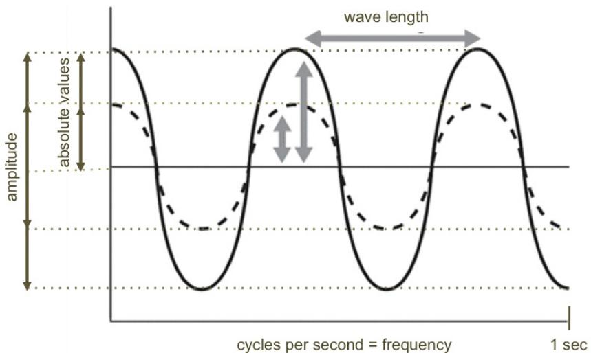
Pitch, i.e. frequency analysis is far more complex than amplitude analysis. Sounds include a range of frequencies (spectral shape), from which the software must extract the fundamental based on mathematical calculations. The question is what the notion of "fundamental" entails.
